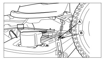
Figure 7. Leveling The Mower Side-to-Side Eccentric Nut Models
